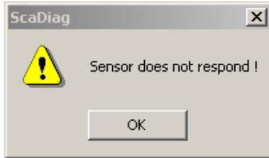
Whenever the tab is switched *ScaDiag* automatically updates the parameter values shown on the new tab. For this purpose, *ScaDiag* tries to set up a communication with the *Scatec*. If the communication fails, the error message *Sensor does not respond* appears. Simply continue by clicking OK but keep in mind, that no data with the *Scatec* can be exchanged!
