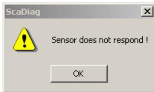
Certain operations (such as tab switching for example) causes *ScaDiag* to communicate with the connected *Scatec*. Failed communication prompts an error message "*sensor does not respond*".
