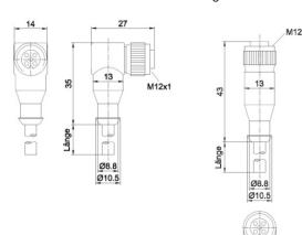
In case of flexible cable installation a minimum bending radius of 5 x  $\varnothing$  has to be observed.
