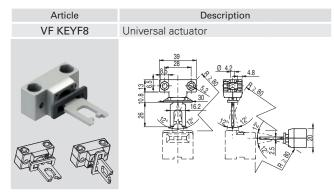
Jointed actuator for guards with poor alignment, adjustable in two dimensions for small doors; can be mounted in various positions. The metal fixing body has two pairs of bore holes; it is provided for rotating the working plane of the actuator by 90°.
