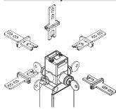
The auxiliary key release device is used to allow the maintenance or the entry into the machinery to authorized personnel only. Turning the key corresponds to actuating the solenoid: the actuator is released. The device can be turned, thereby enabling installation of the safety switch in the machine while the release device remains accessible on the outside of the guard.
