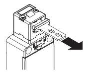
The robust interlocking system guarantees a maximum actuator holding force of  $F_{1max} = 1100 \text{ N}.$
