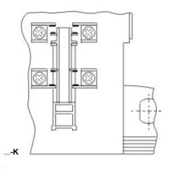
The auxiliary contact K shows the top position of the switch. This enables detecting which guard is unlocked. It is always the top contact.
