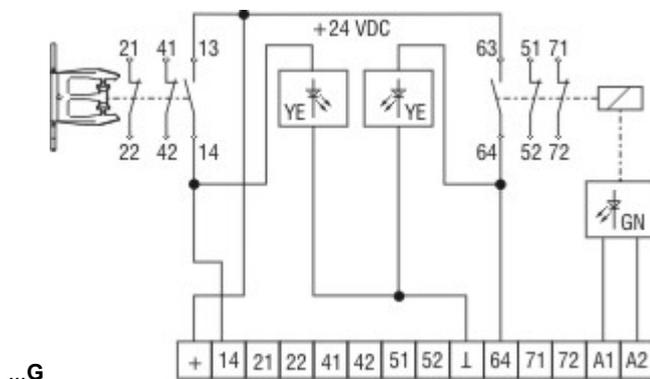
Protected against incorrect polarity and voltage spikes.
