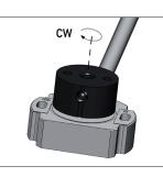
When the marking of the position marker is pointing away from the cable, the output is in the vicinity of the reference pulse (*Z*). Rotational direction CW: A leads before B.
