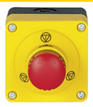
E-STOP/contact block incl. Surface mount housing, set consisting of E-STOP pushbutton with E-STOP symbol and with logo and contact block with monitoring. 2 N/C , with spring-loaded terminals.
