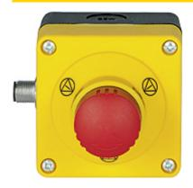
E-STOP/contact block incl. Surface mount housing, set consisting of E-STOP pushbutton with E-STOP symbol and with logo, and contact block, 2 N/C, with M12 connection 5-pin.
