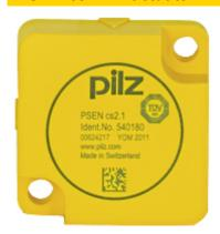
RFiD safety switch 2 safe semiconductor outputs, 8-pin M12 connector, four directions of actuation IP67, operating distance 21 mm, Sao = 15 mm, Sar = 40 mm, PU = 1 piece actuator A total of 8 learning procedures are possible.
