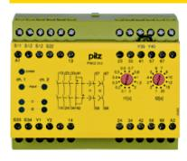
Safety relay (standalone) Inputs: 1-/2-channel wiring with/without detection of shorts across contacts. Outputs:  $3\ N/O$ ,  $1\ N/C$ ,  $2\ N/O$  delayed UB -24 V DC (Japan), width: 112.5 mm, integral screw terminals Monitoring E-STOP, safety gates with two freely selectable delay-on de-energisation contacts, 12 stages from  $0 - 20/0 - 3\ s$ .
