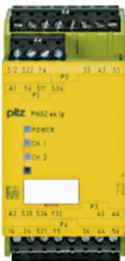
Safety relay (standalone) Inputs: 1-/2-channel wiring with/without detection of shorts across contacts Outputs: 2 safety outputs + 1 auxiliary output in semiconductor technology, 4 N/O Automatic/monitored start, UB 24 V DC, width: 45 mm, plug-in Terminals of screw type, connecting several devices, Monitoring E-STOP, safety gates.
