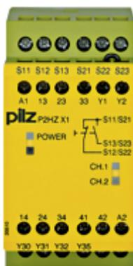
Safety relay (standalone) Inputs: 1 N/O, 1 N/C per pushbutton Outputs: 3 N/O, 1 N/C, 2 semiconductor UB 240 V AC, width: 45 mm, plug-in terminals of screw type Two-hand control device, monitoring the simultaneity of two-hand pushbuttons.
