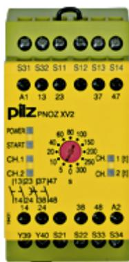
Safety relay (standalone) Inputs: 1- / 2-channel wiring with detection of shorts across contacts Outputs: 2 N/O, 2 N/O delayed UB 24 V DC, width: 90 mm, plug-in terminals of screw type Monitoring E-STOP, safety gates with 2 delay-on de-energisation contacts. Release time 12 stages from 0 - 300 s.
