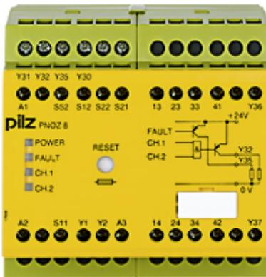
Safety relay (standalone) Inputs: 1-/2-channel wiring with/without detection of shorts across contacts Outputs: 3 N/O, 1 N/C, 2 semiconductor UB 24 V DC, width: 90 mm, plug-in terminals of screw type Monitoring E-STOP, safety gates.
