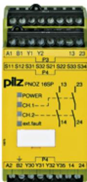
Safety relay (standalone) Inputs: 1-/2-channel wiring with detection of shorts across contacts Outputs: 2 N/O, 2 semiconductor. Automatic/manual reset UB 230V AC/24 V DC, width: 45 mm, plug-in terminals of screw type Monitoring E-STOP, safety gates.
