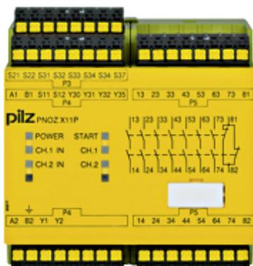
Safety relay (standalone) Inputs: 1-/2-channel wiring with/without detection of shorts across contacts Outputs: 7 N/O, 1 N/C, 2 semiconductor. Automatic/monitored start UB 230 - 240 V AC, width: 90 mm, plug-in spring-loaded terminals Monitoring E-STOP, safety gates.
