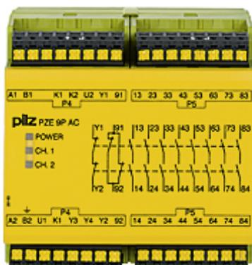
Contact expansion Inputs: 1-/2-channel wiring with/without detection of shorts across contacts Outputs: 8 N/O, 1 N/C. UB 24-240 V AC/DC, width: 90 mm, plug-in spring-loaded terminals.
