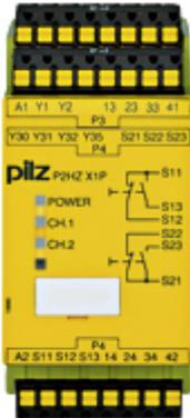
Safety relay (standalone) Inputs: 1 N/O, 1 N/C per pushbutton Outputs: 3 N/O, 1 N/C, 2 semiconductor. UB 42 V AC, width: 45 mm, plug-in spring-loaded terminals. Two-hand control device/monitoring the simultaneity of two-hand pushbuttons.
