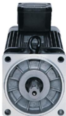
with brake; Feedback system Hiperface multi-turn Resolution of 4096 revolutions with 512 steps each  $M_o = 0.80 \text{ Nm}$   $I_o = 1.10 \text{ A}$   $U_N = 400 \text{ V}$   $n_N = 6000 \text{ min}^{-1}$   $J_{mot} = 0.35 \text{ kgcm}^2$  only suitable for PMC servo controllers (DD5, protego D).
