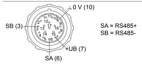
At the tee connector M23, the power supply for the encoder is not connected to the WLAN adapter (pin 7 + 10 are not connected).
