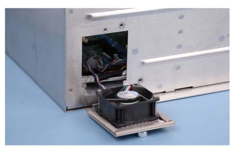
Disconnect the supply cable from the motherboard. Therefor it can be necessary to remove the housing cover.
