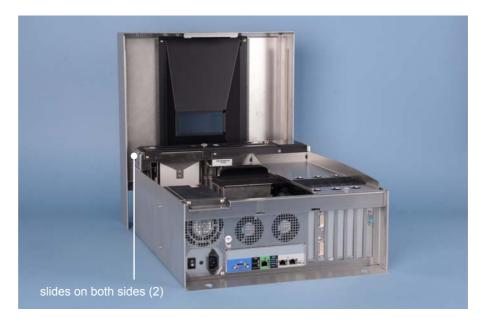
Now the housing cover can be taken off completely, so providing access to the components.
