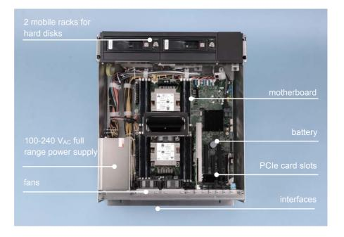
Under the housing cover there is a motherboard with two Intel® Xeon® prozessors with each 6, 12 or 18 Cores.
