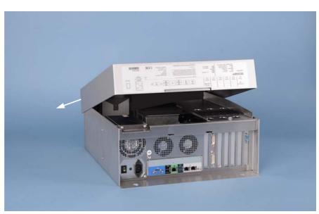
After folding up the cover as shown, it can be pulled out of the slides in direction of the arrow.
