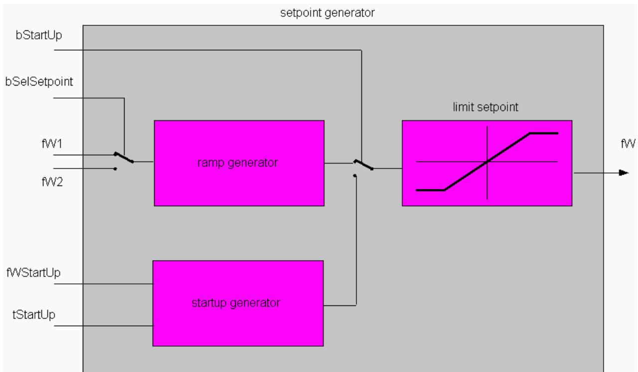
In order to permit "heater baking", a soft start can be parameterised. In this case, the temperature is first ramped up from ambient to a low set value (fWStartUp). This temperature is then maintained for a period of time (tStartUp), and only after that has elapsed does the ramp up to the actual set value begin.
