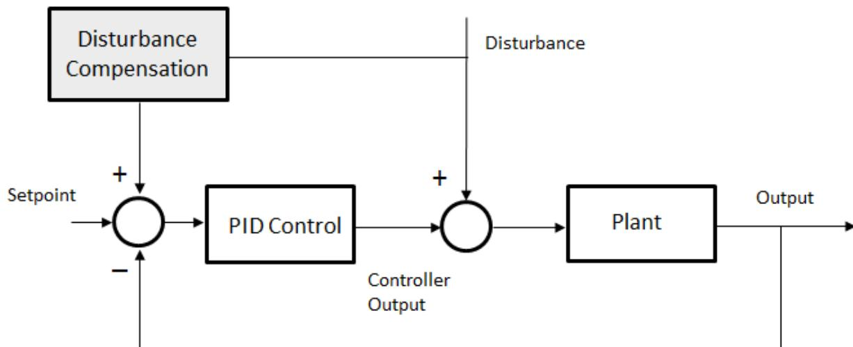
The disturbance compensation is actually a Lead-Lag compensator. A Lead-Lag compensator is a versatile component, which can be used to achieve I, D, PI, PD and PID type compensators by carefully choosing its gain and time constants. The compensator is useful to reduce steady state error, peaks, and improving the dynamic response to the disturbance. More information about the Lead-Lag compensator can be found [here](#).
