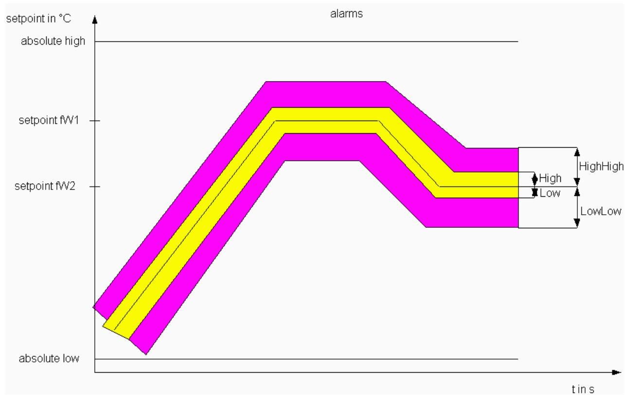
The following alarm conditions are continuously monitored by the temperature controller:
