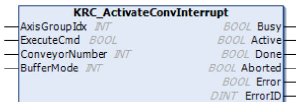
Fig. 43: Function block KRC_ActivateConvInterrupt
