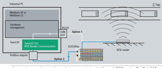
A separate connection must be made to a separate terminal for each RFID reader. The TwinCAT RFID library does not support multiple RFID readers on the same RS485 network for the time being.
