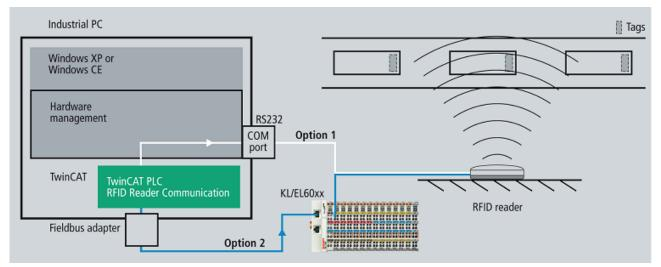
Handling of the library is the same for all supported RFID reader models. In the event of a change of manufacturer, only minor changes to the application are required.
