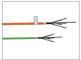
Orange cables (power) and green cables (feedback) are used for the connection between motor and servo drive.
