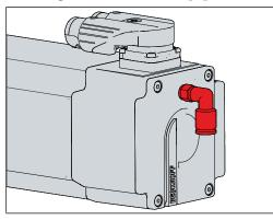
Ingress of liquids or dust at different temperature ranges can be prevented by a separate sealing air connection [+]. It is installed together with an axial shaft seal ring. A defined overpressure is created during assembly.
