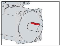
The motors are available with feather key groove and fitted feather key [+] according to DIN6885. The rotor is balanced with half a feather key [+] (according to DIN ISO 21940-32:2012-08).
