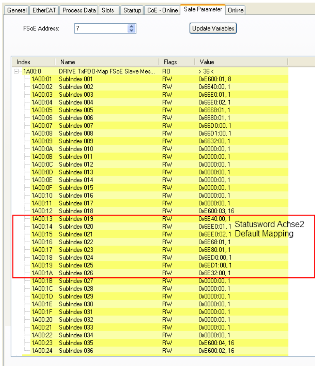
Fig. 19: Status word default mapping for axis 2
