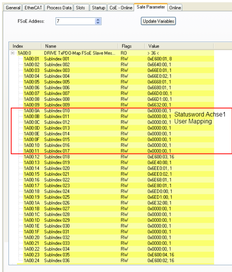
Fig. 18: Status word user mapping for axis 1
