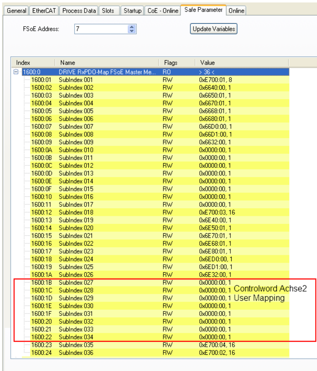
Fig. 16: Control word user mapping for axis 2
