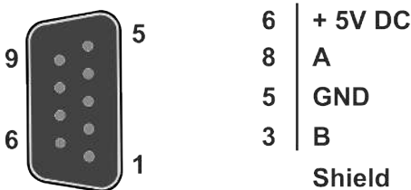
Fig. 20: Pin assignment of the PROFIBUS D-sub socket
