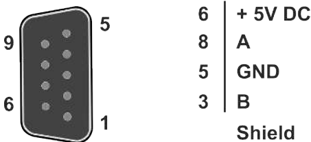
Fig. 20: Pin assignment of the PROFIBUS D-sub socket
