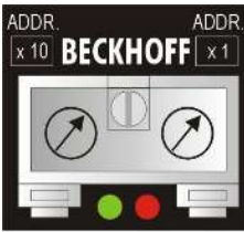
Fig. 141: Address selection switch
