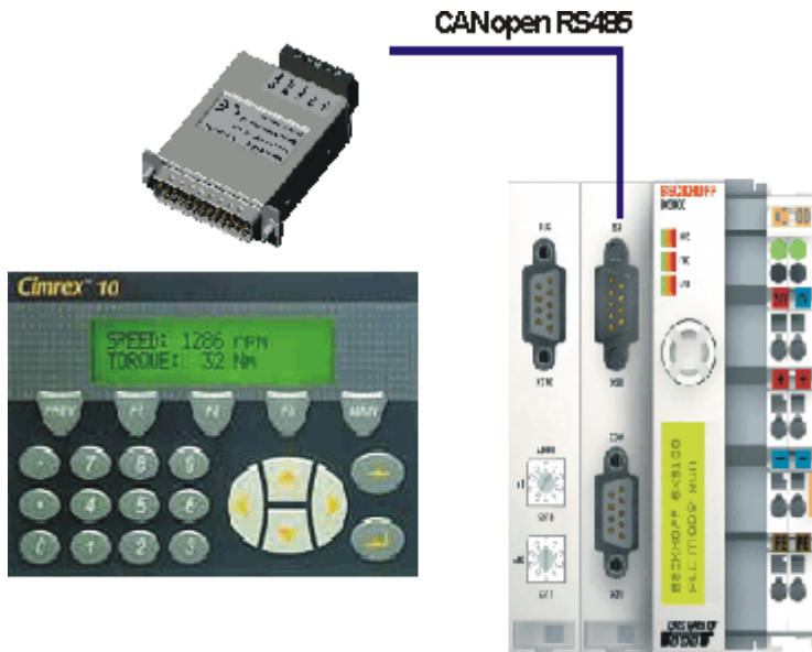
Fig. 75: Cimrex panel at the SSB of the BX controller
