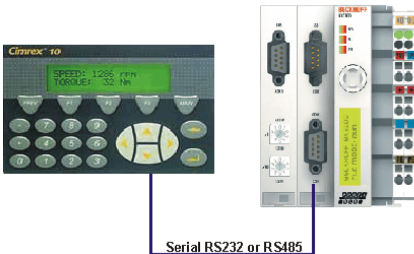
Fig. 120: Cimrex panel at the COM port of the BX controller
