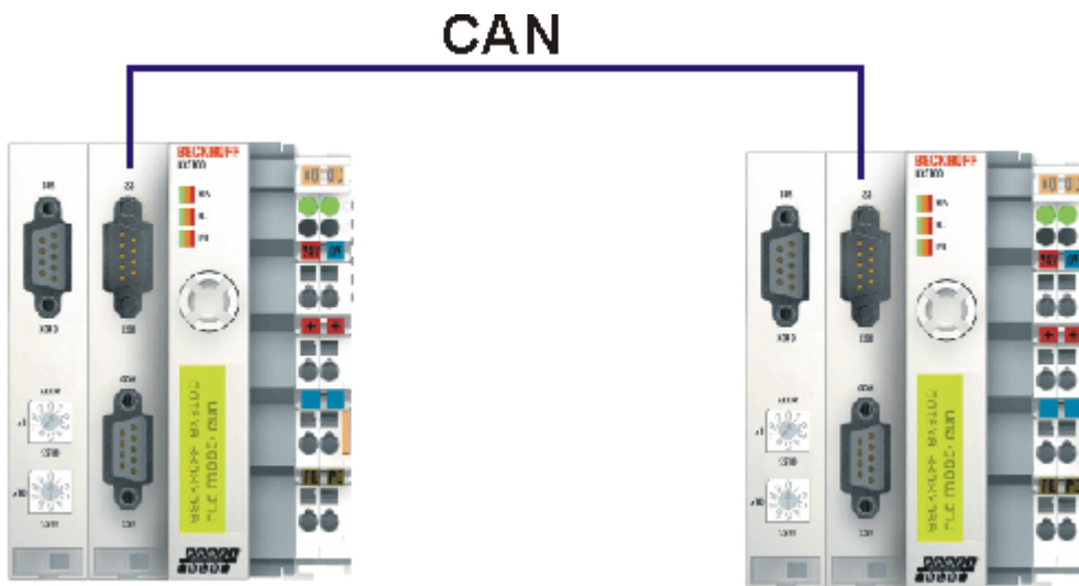
Fig. 72: Communication between BX controllers (via SSB)
