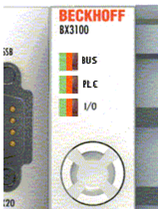
Fig. 144: Diagnostic LEDs for the fieldbus, the PLC and the K-bus
