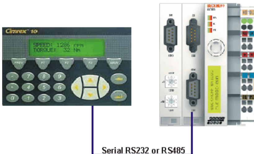
Fig. 107: Cimrex panel at the COM port of the BX controller
