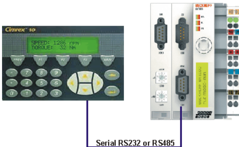
Fig. 124: Cimrex panel at the COM port of the BX controller
