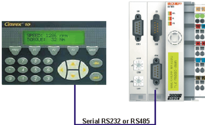
Fig. 106: Cimrex panel at the COM port of the BX controller
