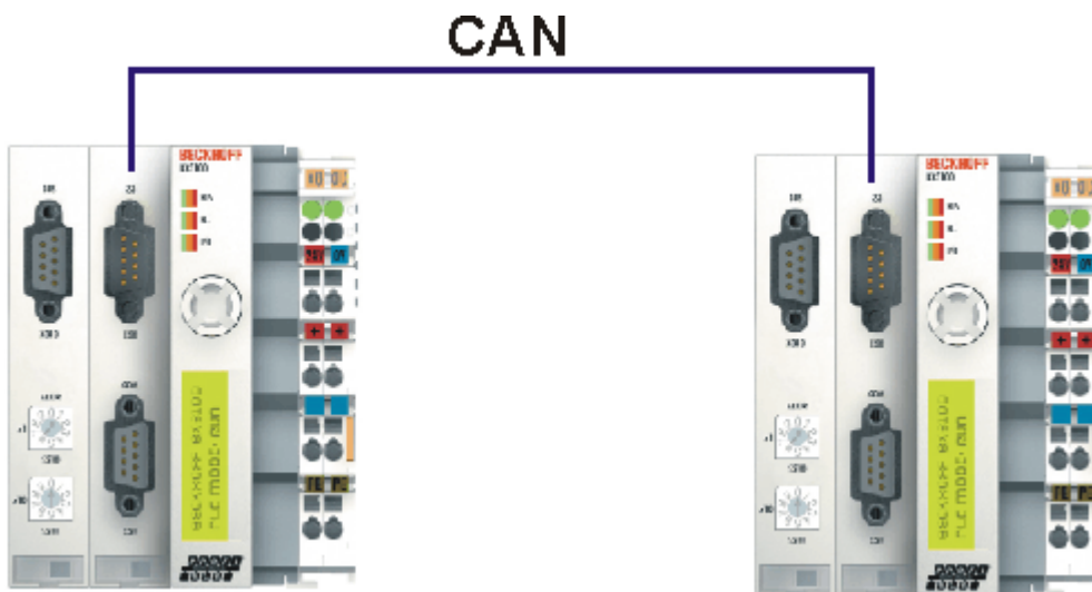
Fig. 58: Communication between BX controllers (via SSB)
