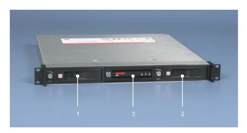
The C5210 is fitted with two removable frames for hard disks (1) and (2). In condition of delivery one of the removable frames is fitted with a hard disk. Behind the flap (3) the control elements and two USB-interfaces are located.
