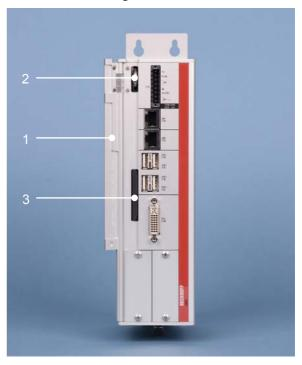
Opening the front flap (1) allows access to the battery (2) and the CFast-Card (3).
