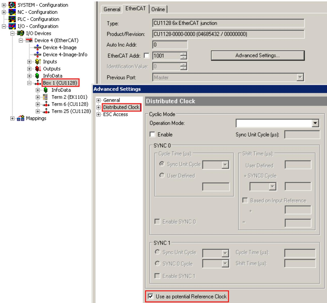
Fig. 94: activating the CU1128 DC function
