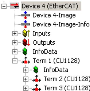
Fig. 101: added CU1128 with secondary devices Dev A and Dev B
