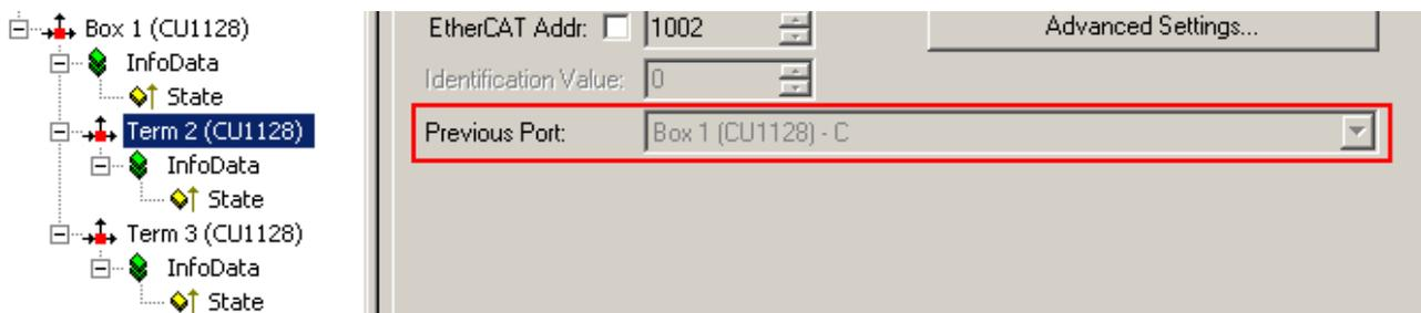
Fig. 11: previous port of the second ESC in the CU1128
