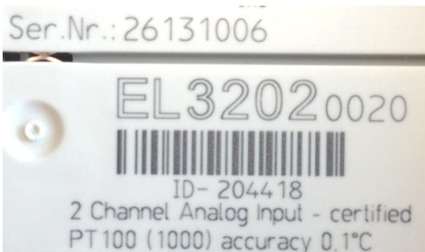
Fig. 4: EL3202-0020 with batch numbers 26131006 and unique ID-number 204418
