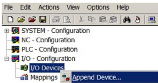
Fig. 42: Append EtherCAT device
