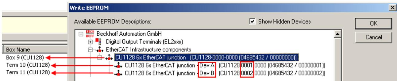
Fig. 114: currently available EEPROM descriptions for CU1128 and assignment
