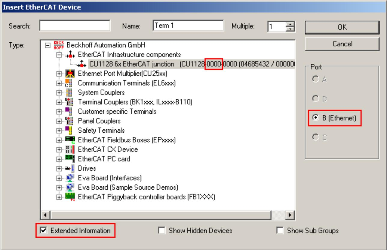
Fig. 100: selection of the main device CU1128-0000
