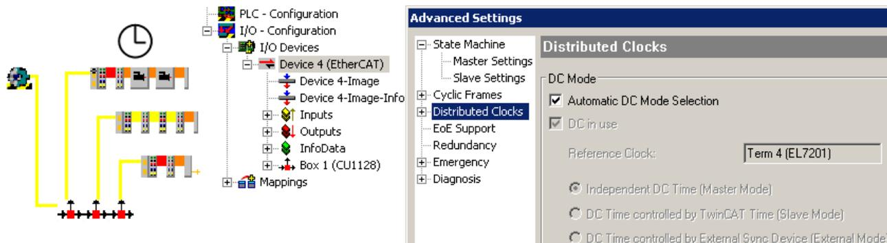
Fig. 93: example topology with EL7201 as reference clock
