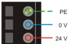
Fig. 23: Pin configuration of the spring loaded terminal
