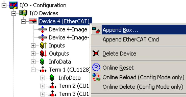
Fig. 104: adding further CU1128 devices
