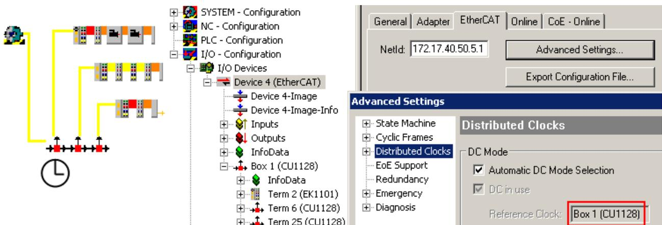
Fig. 95: CU1128 as reference clock
