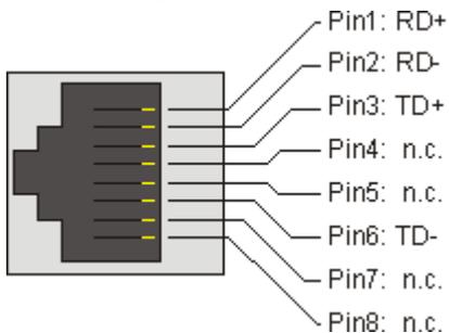
Fig. 24: Pin configuration of the RJ45 sockets
