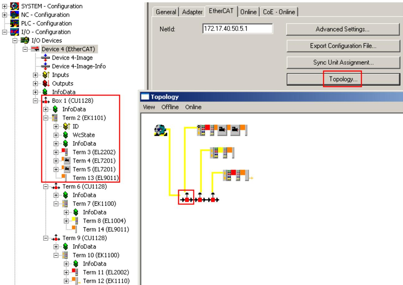
Fig. 97: CU1128 topology display in the System Manager
