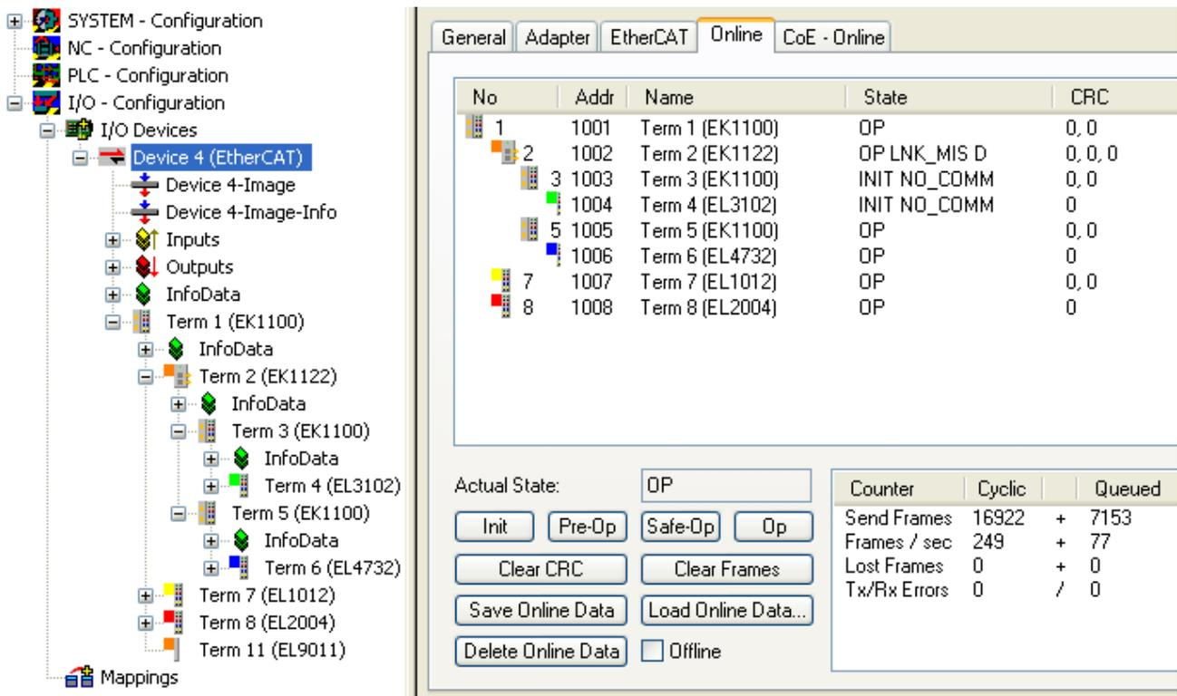
Fig. 18: Example configuration with interrupted cable
