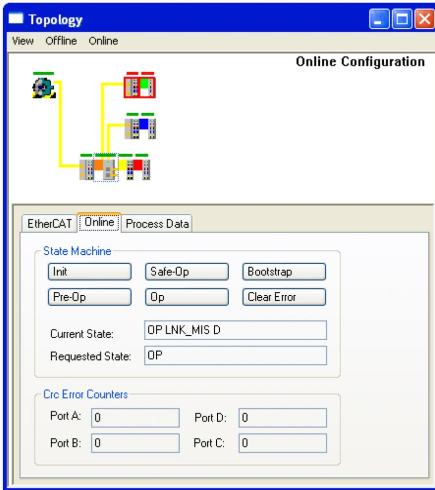
Fig. 19: Topology display for interrupted line
