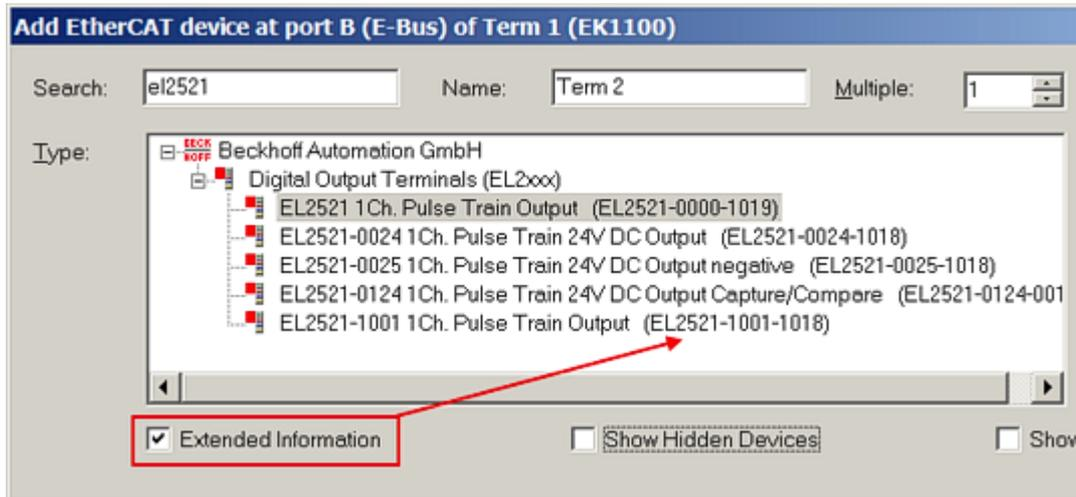
Fig. 49: Display of device revision
