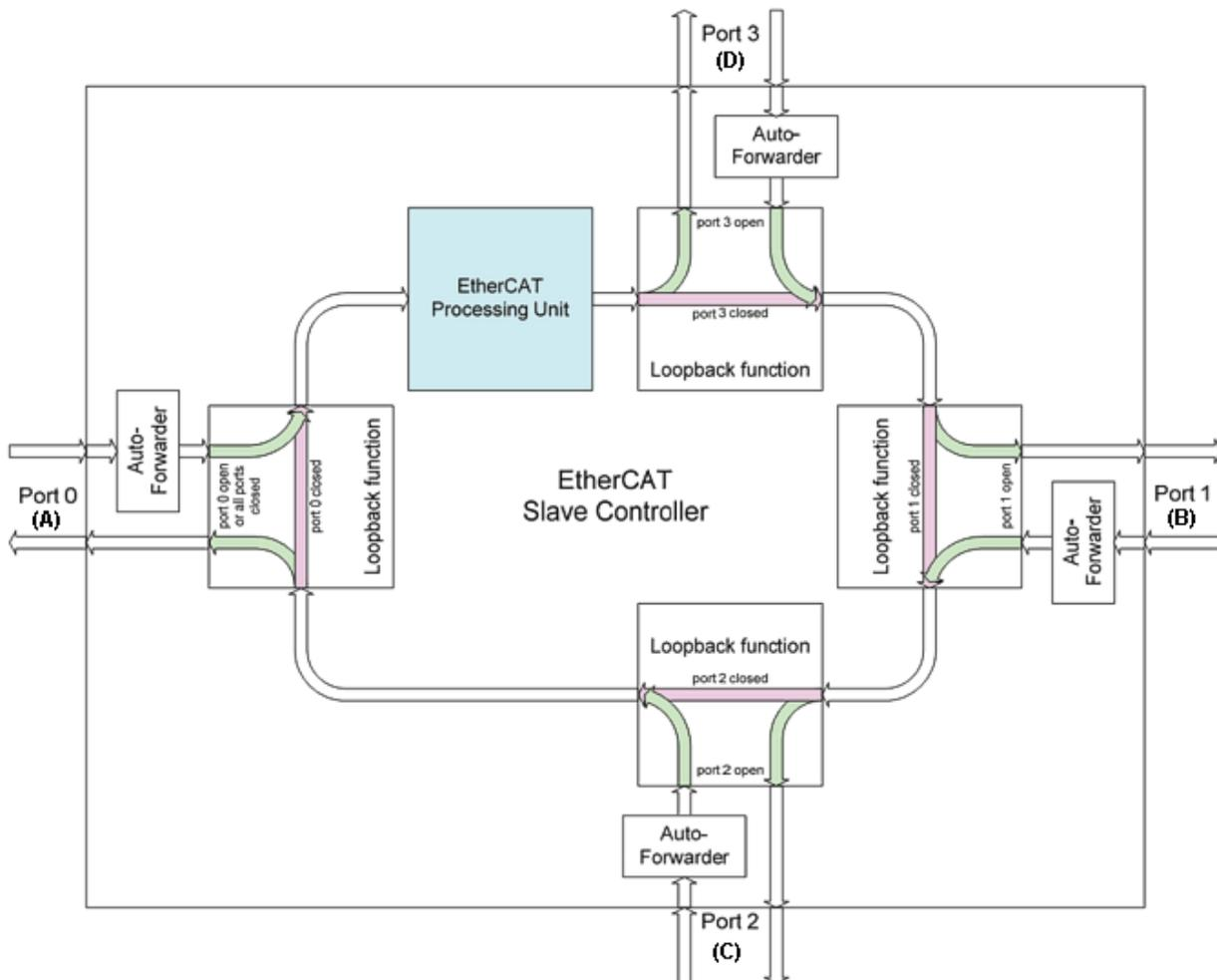
Fig. 15: Direction of data flow in the ESC
