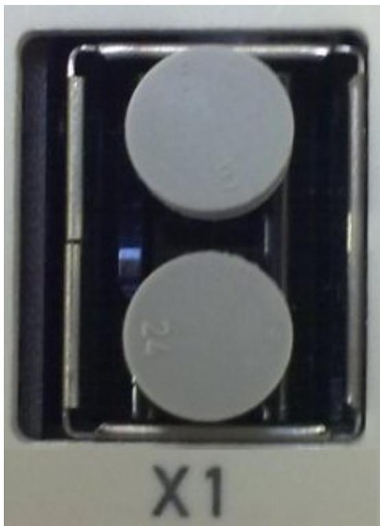
Fig. 30: Blind plugs in unused sockets
