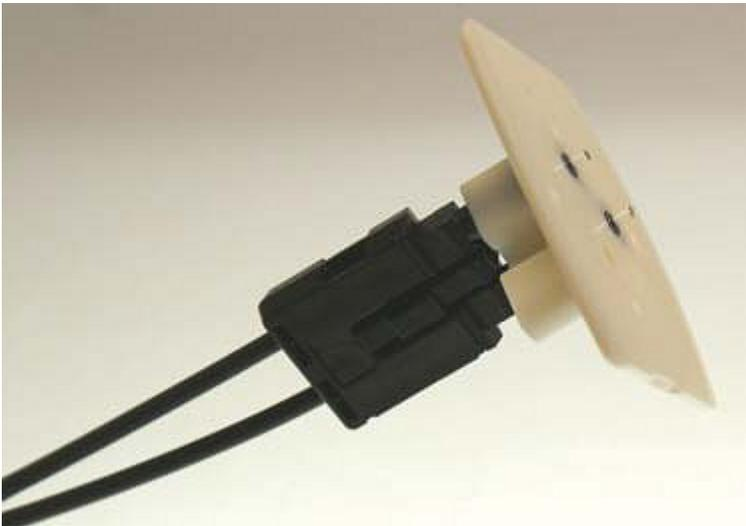
Fig. 36: Sanding gauge with protruding fiber ends
