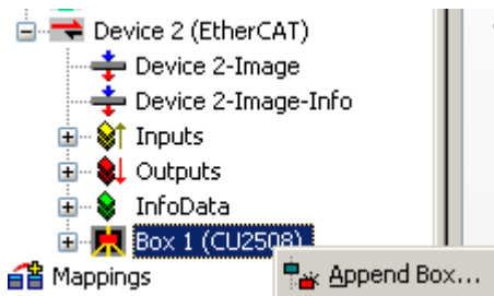
Fig. 38: Appending further EtherCAT slaves
