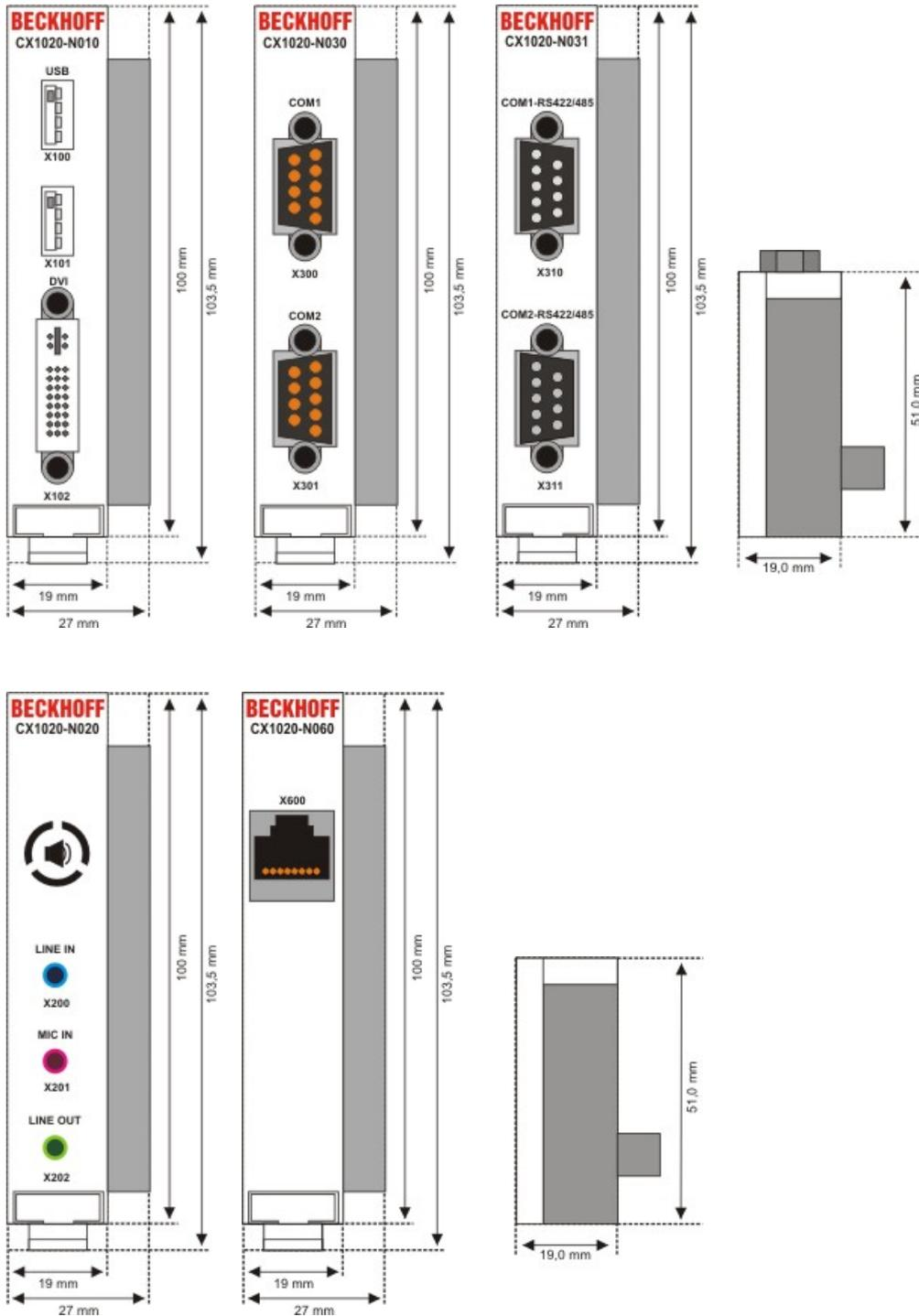
Like for the CX1000, a number of optional interface modules are available for the basic CX1020 CPU module that can be installed ex works. The following interfaces are available:
