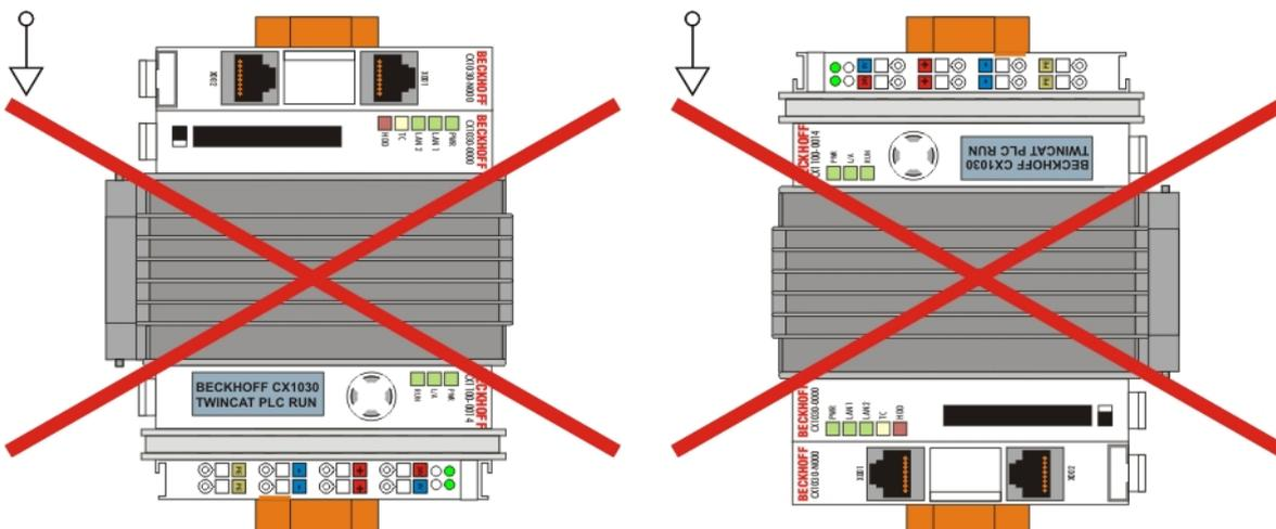
The installation position "backside down" is only allowed with the right power supply. The power supply should have a cooling plate (CX1100-001x).
