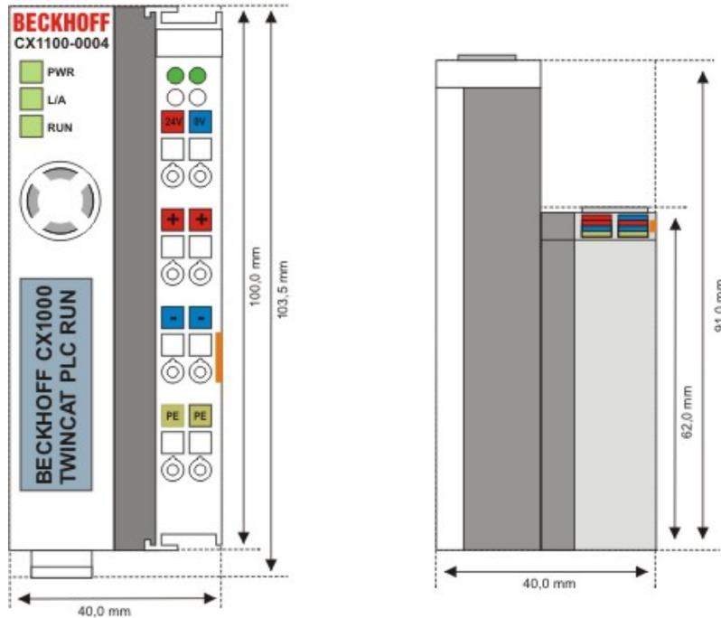
With the CX1100-0004 power supply EtherCAT Terminals can be connected to the CX10x0-System. With CX1100-0004 the I/O data are stored directly in the main memory of the CPU; a DPRAM is no longer required. The CX1100-0004 power supply unit for EtherCAT Terminals can not be connected in conjunction with the basic CX1000 CPU module.
