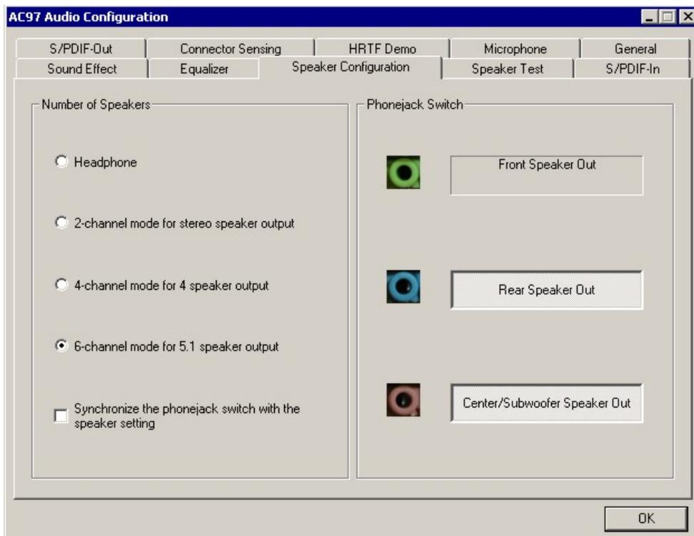
The colours of the connections shown match those on the CX1020-N020 module. Once a configuration has been set it can be tested via the **"Speaker Test"** tab.
