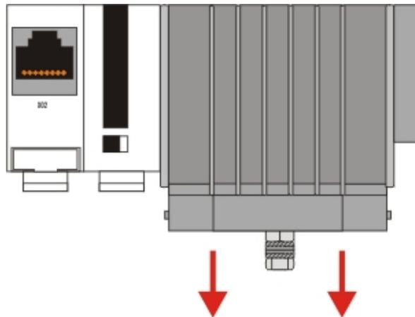
**3. Take the cartridge towards the front. The cartridge is now removed.**
