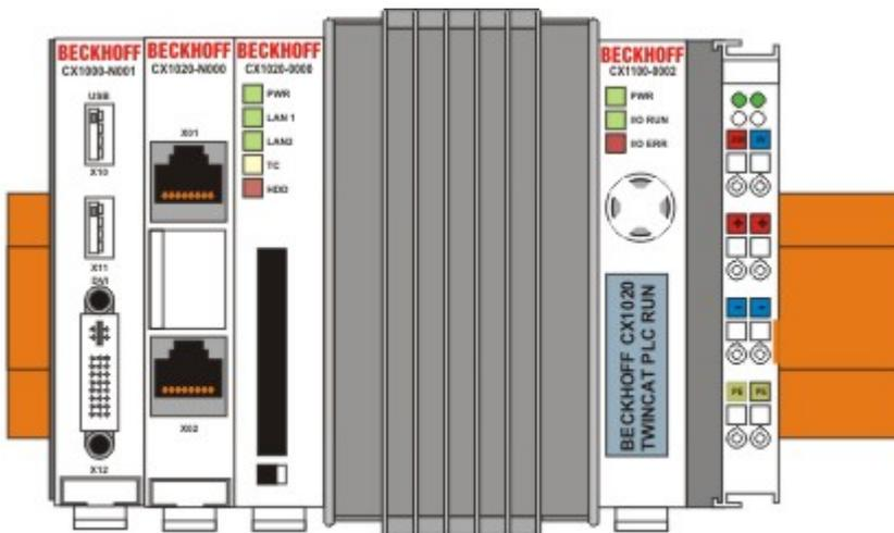
Then fix the CX1020 block on the top hat-rail using the latching straps. You should hear a soft click.
