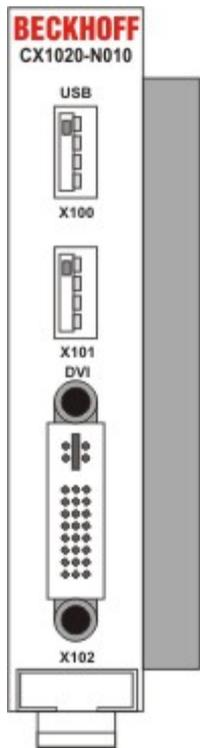
In addition to the two Ethernet interfaces, this module features a DVI-I and two USB interfaces.
