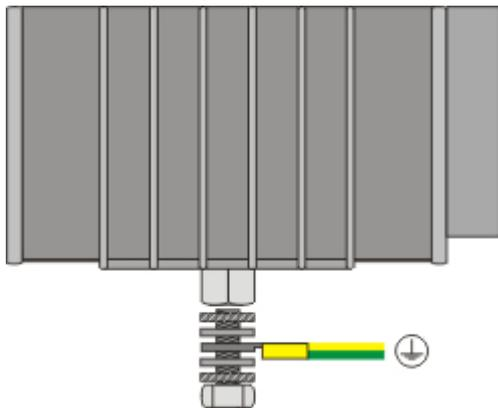
The lug is placed between the middle grommets. First the screw is fixed by turns with the hand. Then a wrench of size S7 can be used to fix the screw. To avoid damage to the unit, its a good idea to make use of a torque wrench.
