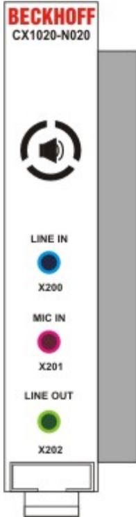
This system interface provides the audio interface for the CX1020 system. Two inputs, "LINE IN" and "MIC IN", are available. The "LINE OUT" connection is used as output for audio signals. It can also be used for connecting headphones with a maximum output of 200 mW. It also features a PC beeper. The audio interfaces are accessed via the operating system. "Windows XPe" offers an option for switching the audio module to surround mode.
