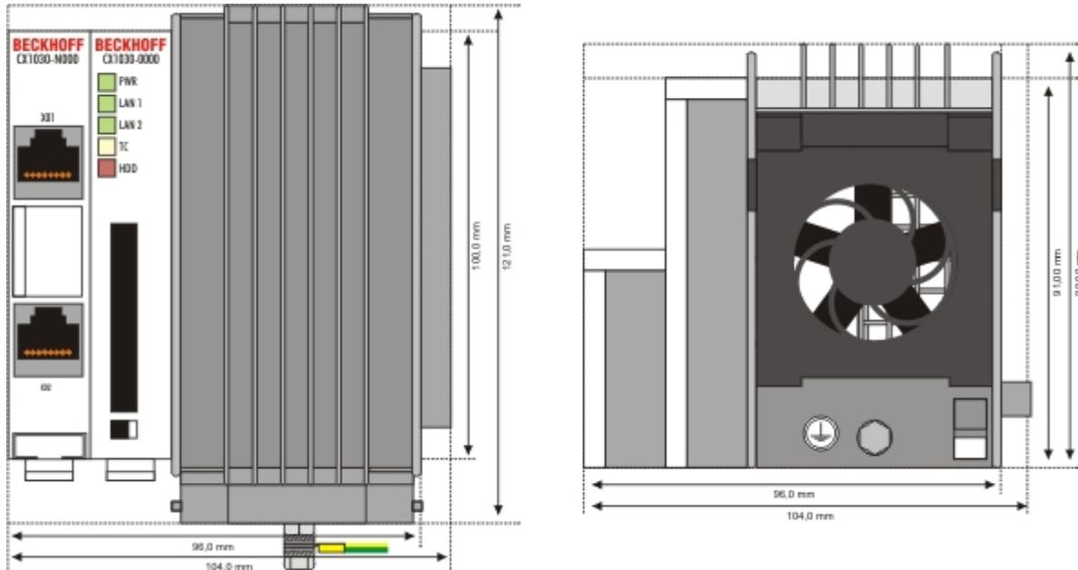
The basic configuration of the CX1030 includes a 64 MB Compact Flash card. Two Ethernet RJ 45 interfaces are also part of the basic configuration. These interfaces are connected to an internal switch and offer a simple option for creating a line topology without the need for additional Ethernet switches. All other CX family components can be connected via the PC104 interface that is available on both sides.
