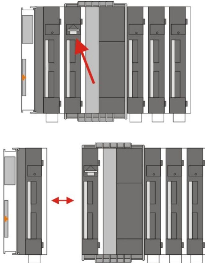
Only modules (CPU, fieldbus connections and UPS modules) that can be separated non-destructively feature a release device. Modules that cannot be separated only feature a marking point (with or without red paint seal). Applying force to these elements will destroy them.
