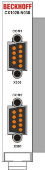
The CX1020-N030 system interface features two RS232 interfaces, COM1 and COM2 (9 pin Sub-D plug connector). If there is need for more than two serial interfaces two further RS232 interfaces, COM3 and COM4 (9 pin Sub-D plug connector) can be added to the system via the system interface CX1020-N40. The maximum baud rate on all channels is 115 kBit. The pin assignment for all interfaces is equal and described below. The interface parameter can be set in the operating system or in the PLC program.
