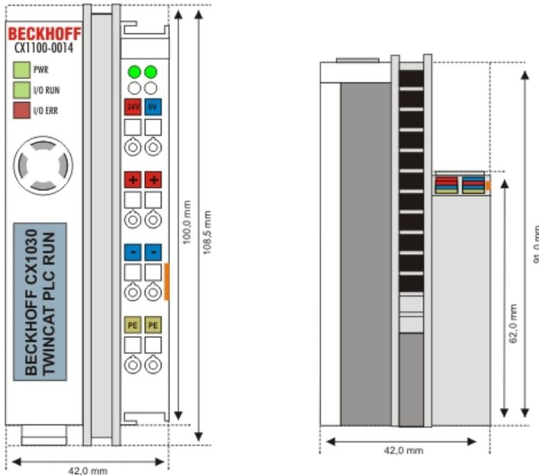
The CX1100-0014 power supply is designed for CX1030.
