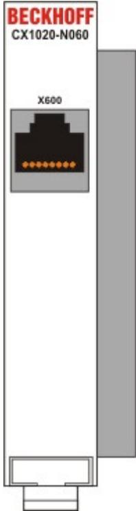
The CX1020-N060 system interface provides a further network interface. It can only be used if the CX1100-0004 power supply unit is not connected, since in this case the only internal interface available is used for connecting the Ethernet port. (Details see Basic module description.)
