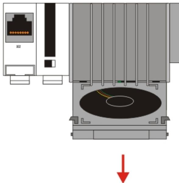
4. Open the packaging of the new fan cartridge and take out the new cartridge. Hold the cartridge in front of the mounting notches. Take care that the notches fit the holes in the back of the housing.
