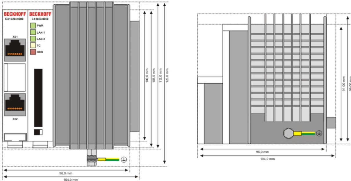
The basic configuration of the CX1020 includes a 64 MB Compact Flash card. Two Ethernet RJ 45 interfaces are also part of the basic configuration. These interfaces are connected to an internal switch and offer a simple option for creating a line topology without the need for additional Ethernet switches. All other CX family components can be connected via the PC104 interface that is available on both sides.
