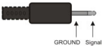
The only existing channel is transferred via the tip, the remainder of the sleeve is used for earthing.
