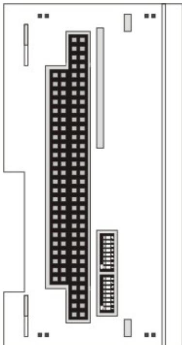
The upper switch sets the parameters for the upper interface, the lower switch sets the parameter for the lower interface. The system must be powered down, if the settings of the switches are changed! The settings for default use should be mentioned by ordering the interface module.
