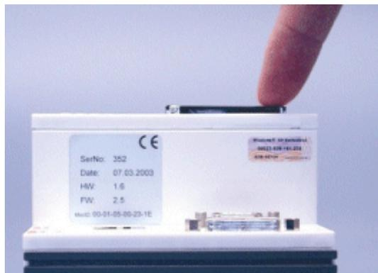
FIG3: Inserting the CF card
