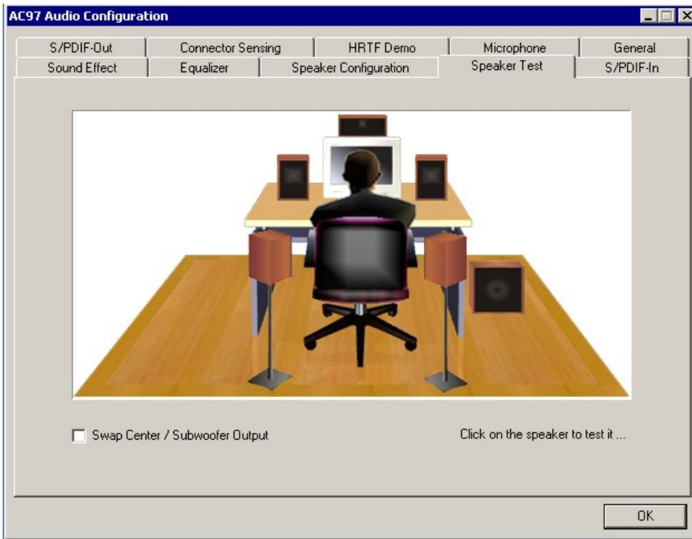
Clicking on a speaker causes a signal to be sent to the selected speaker. The user can thus check the positioning or allocation of the individual speakers to the audio channels. Once all speakers have been set correctly, the surround sound can be tested via **"HRTF Demo"**.
