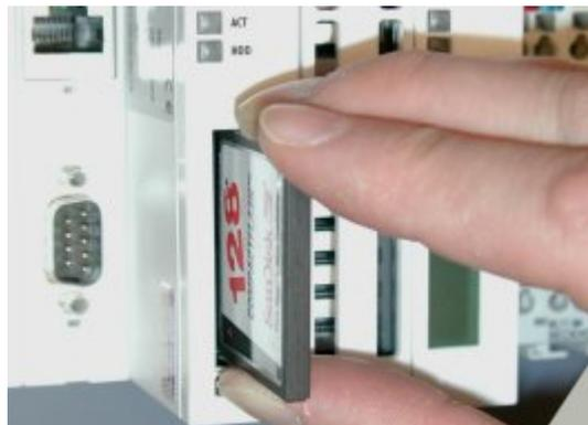
FIG2: Removing the CF card
