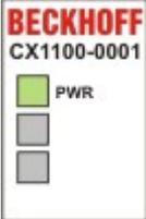
The image shows a close-up of the front panel of a Beckhoff CX1100-0001 power supply unit. It features the Beckhoff logo and model number at the top. Below, there are three indicator LEDs. The top LED is illuminated in green and is labeled 'PWR'. The two LEDs below it are unlit and grey. | Power | The LED lights up green when the power supply is correct, but red if there is a short circuit. |
