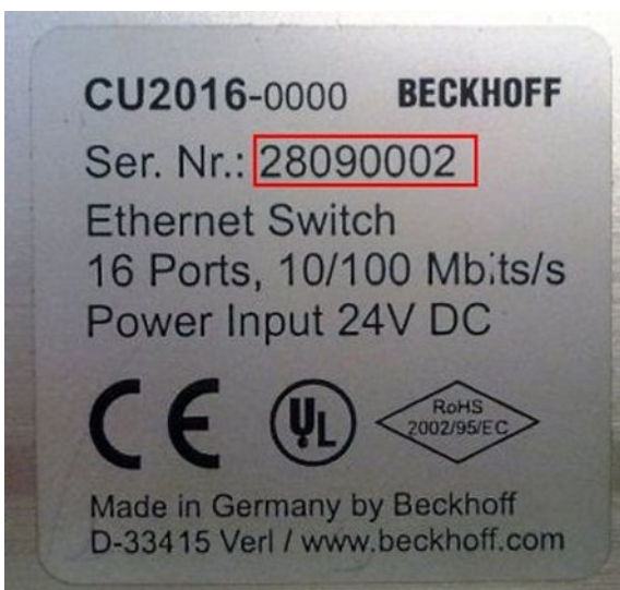
Fig. 3: CU2016 switch with serial/ batch number
