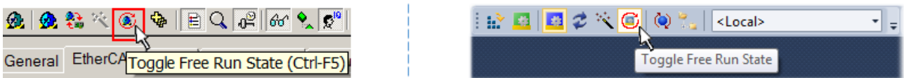
Fig. 107: TwinCAT can also be switched to this state by using a button (left: TwinCAT 2; right: TwinCAT 3)
