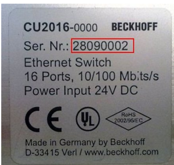
Fig. 3: CU2016 switch with serial/ batch number
