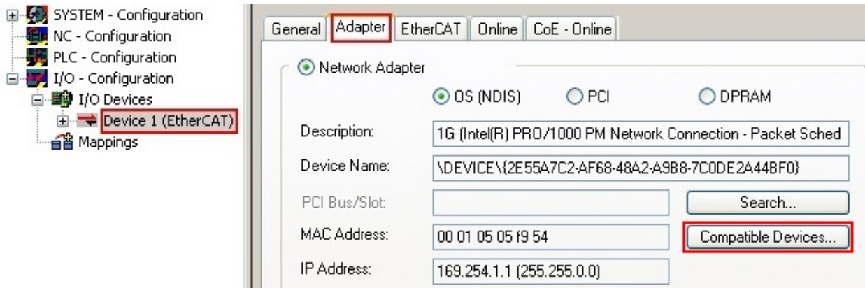
Fig. 72: EtherCAT device properties(TwinCAT 2): click on „Compatible Devices...“ of tab “Adapter”
