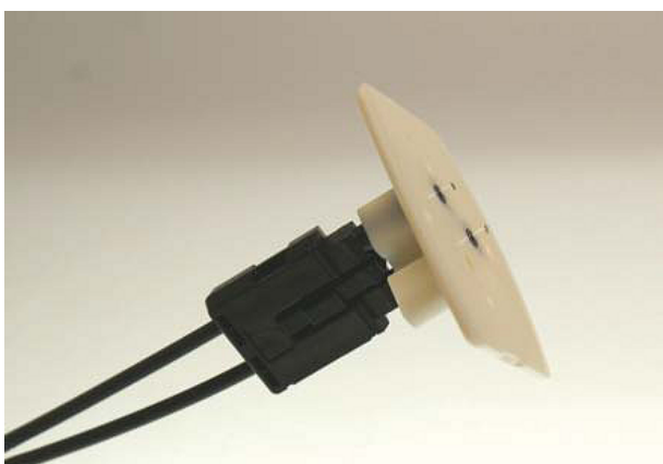
Fig. 54: Sanding gauge with protruding fiber ends
