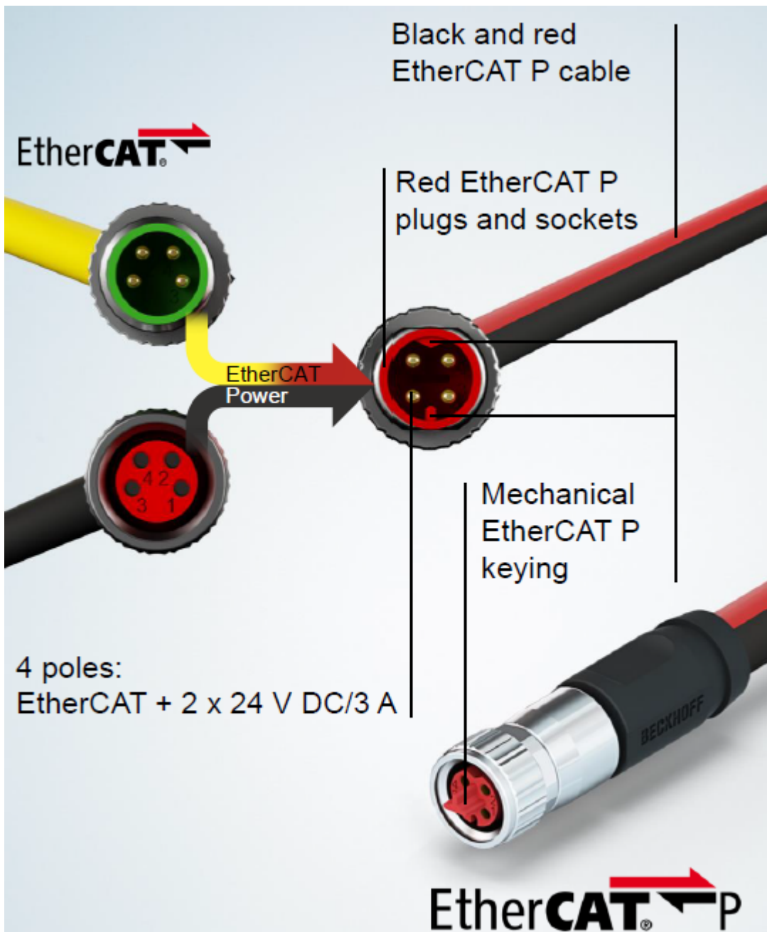
Fig. 13: Connector face: EtherCAT, Power and EtherCAT P
