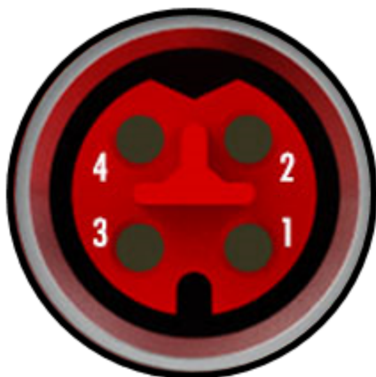
Fig. 29: Pin assignment M8, EtherCAT P In and EtherCAT P Out
