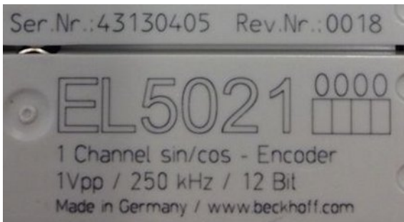
Fig. 1: EL5021 EL terminal, standard IP20 IO device with serial/ batch number and revision ID (since 2014/01)
