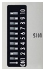
Fig. 18: DIP switch S001: Left off "0", right on "1"
