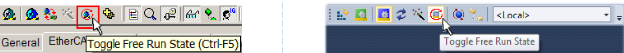
Fig. 108: TwinCAT can also be switched to this state by using a button (left: TwinCAT 2; right: TwinCAT 3)
