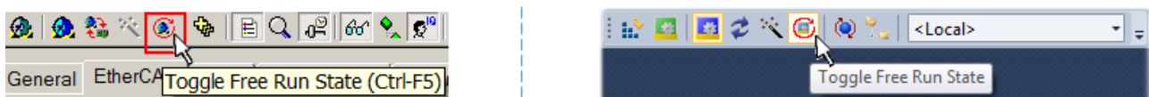
Fig. 105: TwinCAT can also be switched to this state by using a button (left: TwinCAT 2; right: TwinCAT 3)
