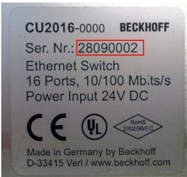
Fig. 3: CU2016 switch with batch number
