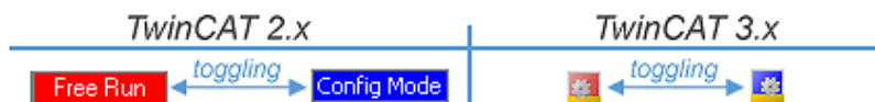
Fig. 103: Displaying of “Free Run” and “Config Mode” toggling right below in the status bar
