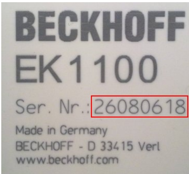
Fig. 2: EK1100 EtherCAT coupler, standard IP20 IO device with batch number
