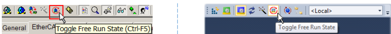
Fig. 60: TwinCAT can also be switched to this state by using a button (left: TwinCAT 2; right: TwinCAT 3)
