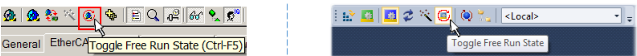
Fig. 164: TwinCAT can also be switched to this state by using a button (left: TwinCAT 2; right: TwinCAT 3)
