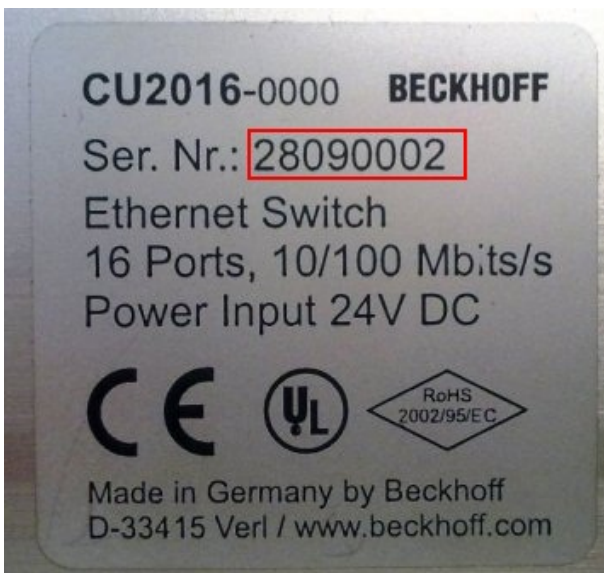
Fig. 3: CU2016 switch with serial/ batch number
